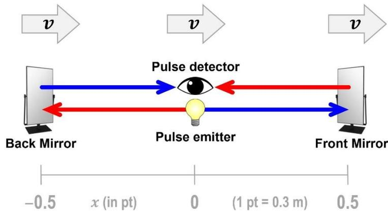
Figure 2. Design of a Javelin Clock
