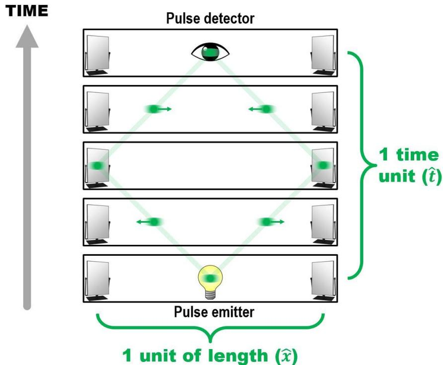
Figure 3. The light pulse paths traced by one cycle of a javelin clock at rest
